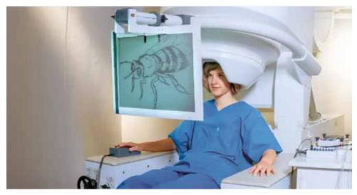
An experiment using magnetoencephalography: the magnetic field generated from brain activity is measured in a female participant integrating visual and acoustic information
